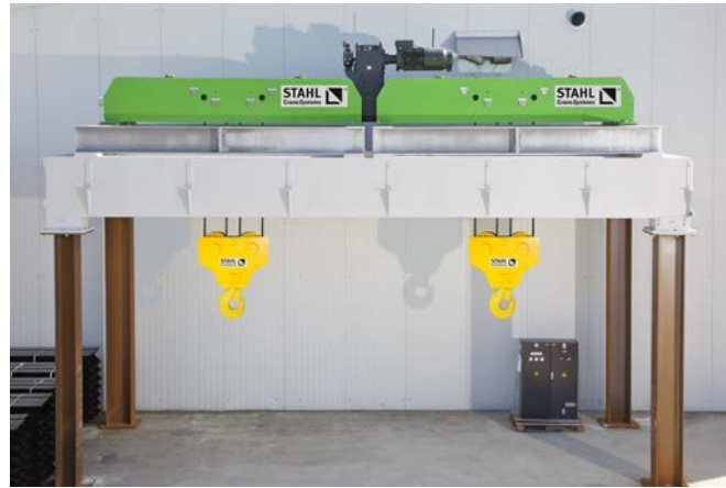
Test set-up of the SHW 8 special winch from STAHL CraneSystems: the gear motor was mounted vertically and the hoist motor above one of the two rope drums.
